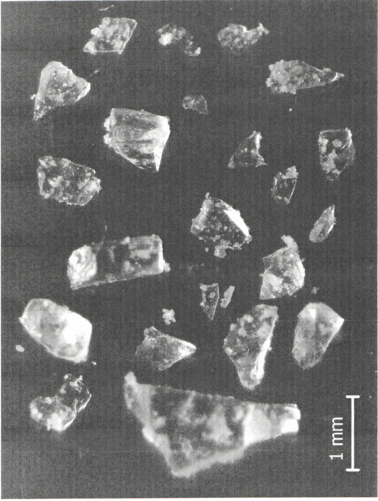
Figure 4. Suspect glass fragments isolated from the complaint sample. Note this does not represent all of the fragments present in the sample.
